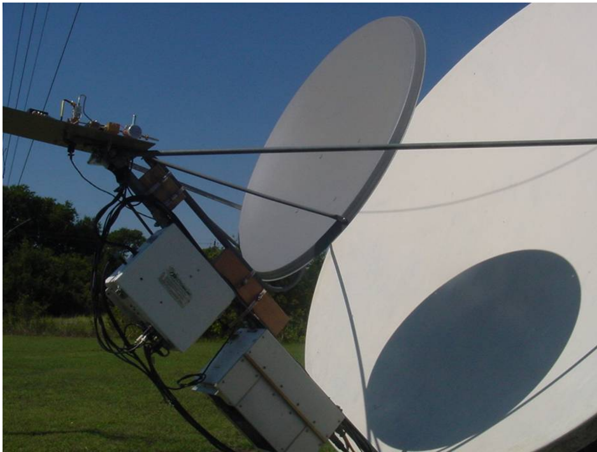
Figure 5 W5LUA 1m Dish Installed on 2.4m Mount
