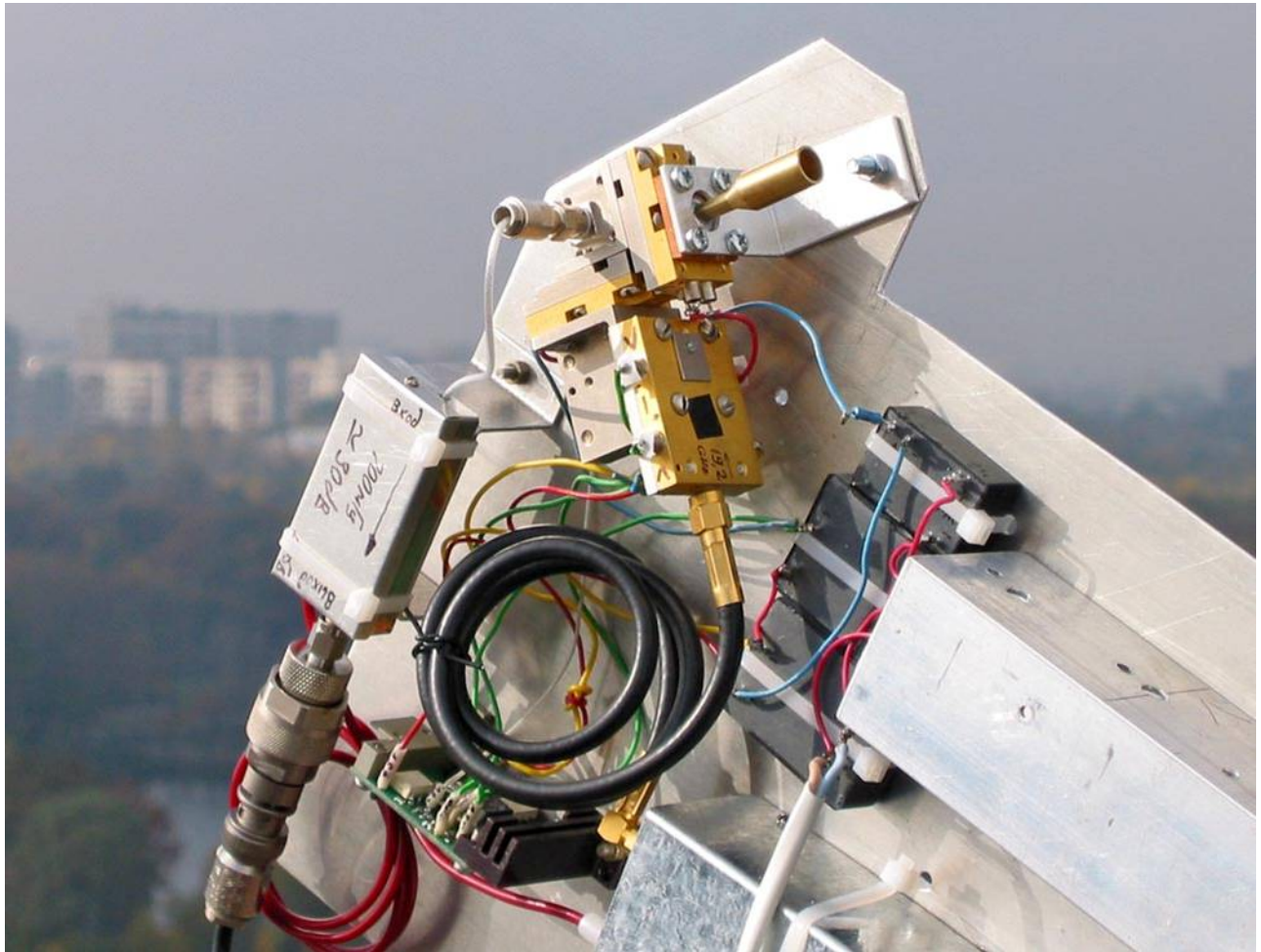
Figure 3 RW3BP 78 GHz RX on 2.4m Dish (2006)
