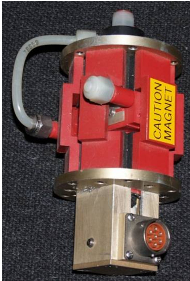
Figure 9 78 GHz 73 W Klystron Tube
